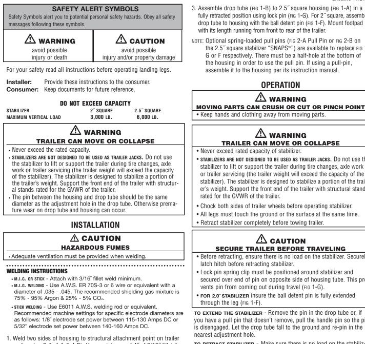
surface (FIG 3-A, 4-A & 4-B). Use a minimum of 4" of 3/16" fillet linear weld total on each side, stich or continuous (FIG 4-A & B). See welding instructions. When locating housing on trailer make sure access for lock pin is available for easy adjustment.
